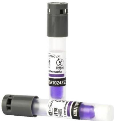
Spore carrier: polyethylene fibers. 17 mm of diameter, 64.5 g/m<sup>2</sup>.  $\geq 10^6$  *Geobacillus stearothermophilus* ATCC®\* 7953 spores per vial. Final fluorescence reading is performed after 5 minute-incubation at 60 °C (sensitivity  $\geq 97\%$ ).
