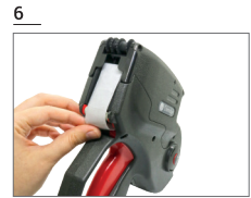
6 Insert the end of the liner into the slot by pressing the trigger | Inserte el extremo del liner en la ranura presionando el gatillo.
