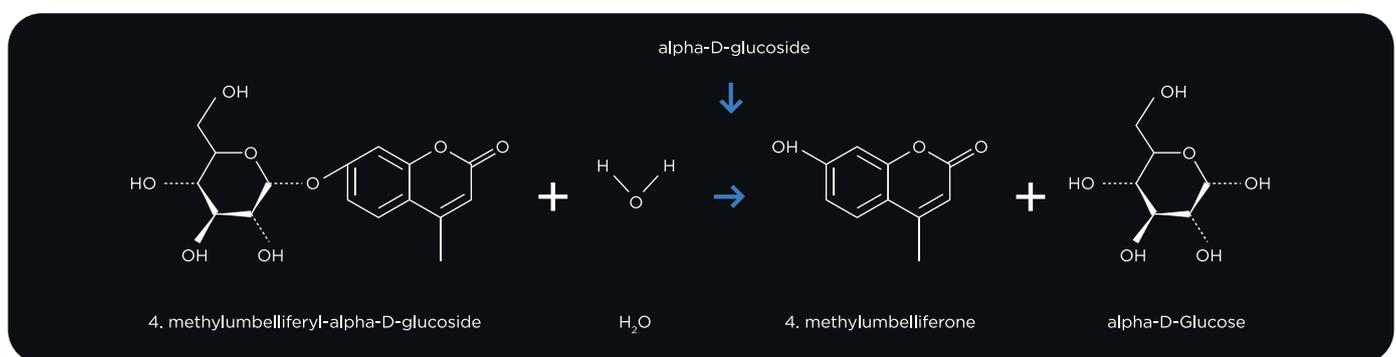
In this way, only these SCBI with viable spores can give a detectable fluorescence signal. Those with dead or inactivated spores will not catalyze that reaction and therefore generate that fluorescent signal.
