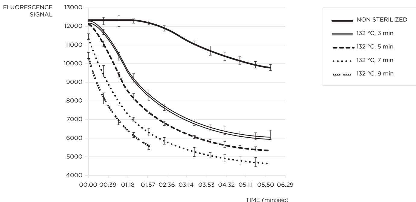
In the graph, we can observe a marked difference between the fluorescent signal of unexposed indicators and the signal of those exposed to different sterilization cycles. **The 7-second reading time with Photon allows maximizing monitoring safety with unprecedented speed.**
