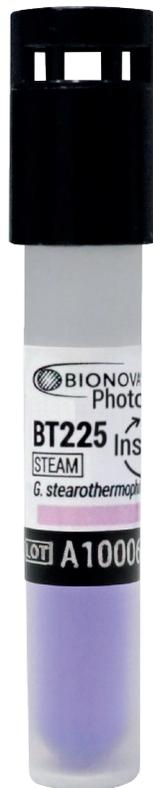
proteins associated with the spore by fluorescence readouts. The transformation of these proteins is directly related to the conditions of the sterilization cycle.
